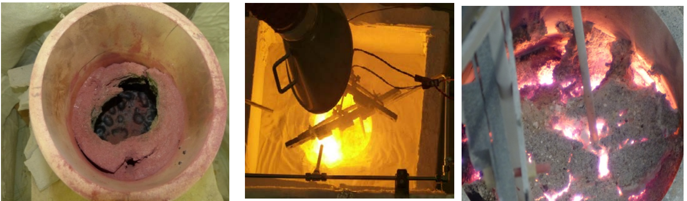
Figure 1 Manufacturing of In and Ex vessel simulants in Plinius facility [4]
